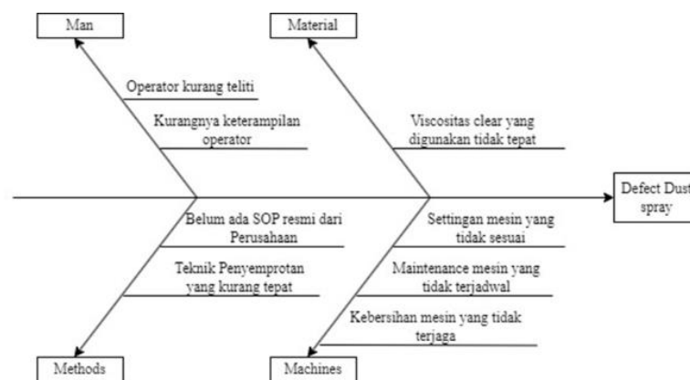
Gambar 2. Fishbone diagram defect dustspray
